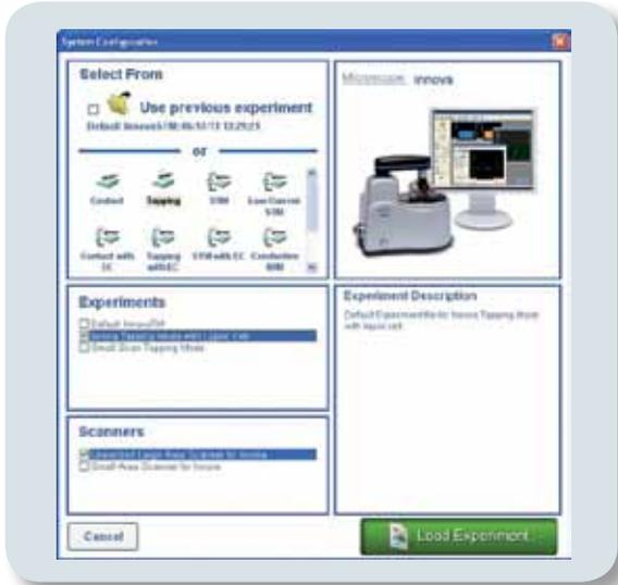
The experiment selector completely preconfigures the system for a wide range of selectable experiments. It is ideal for multi-user settings. The sophistication of the predefined experiments offers beginners a fast path to expert results, while at the same time advanced users can define and save specific configurations exclusively for their own use.
